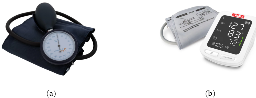
Figure 4.2: Types of sphygmomanometers:(a) Aneroid 1 ; (b) Digital 2
