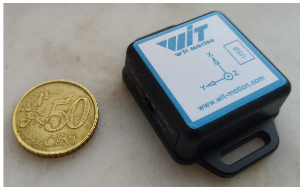
Figure 4.18: WitMotion WT901BLECL BLE5.0
