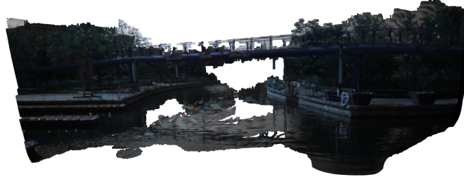
FIGURE 3.14: Dense scene reconstruction from the computed disparity map in a 3D point cloud.
