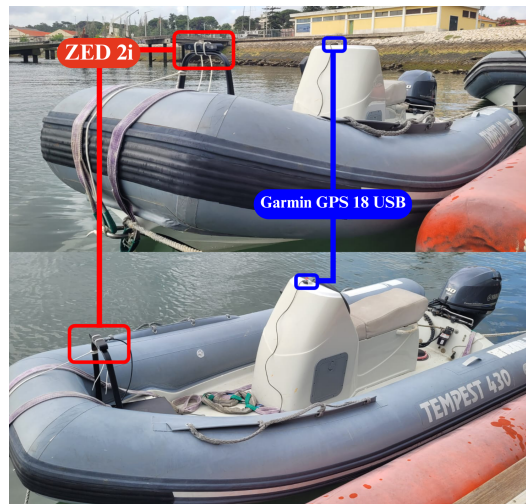
FIGURE 3.9: RHIB setup for dataset capture in the maneuvering basin of the Lisbon Naval Base.
