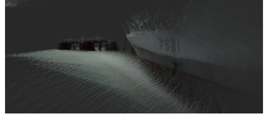
(B) Floating 3D view of the captured vessel and pier in the generated point cloud.
