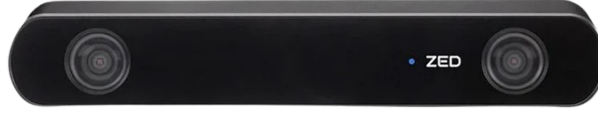
FIGURE 3.4: ZED 2i Stereo Camera (StereoLabs 2024).
