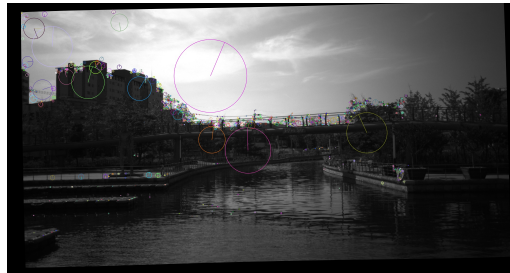
FIGURE 3.15: SIFT keypoints represented with scale and orientation on the left rectified image.
