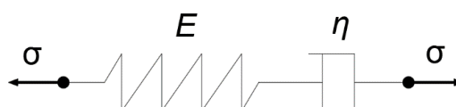
Figura 2.11 – Modelo de Maxwell (adaptado de (Findley.W.N, Lai.J.S, Onaran, K., 1976; Lubarda, 2019; Rajagopal, June 1, 2000)).
