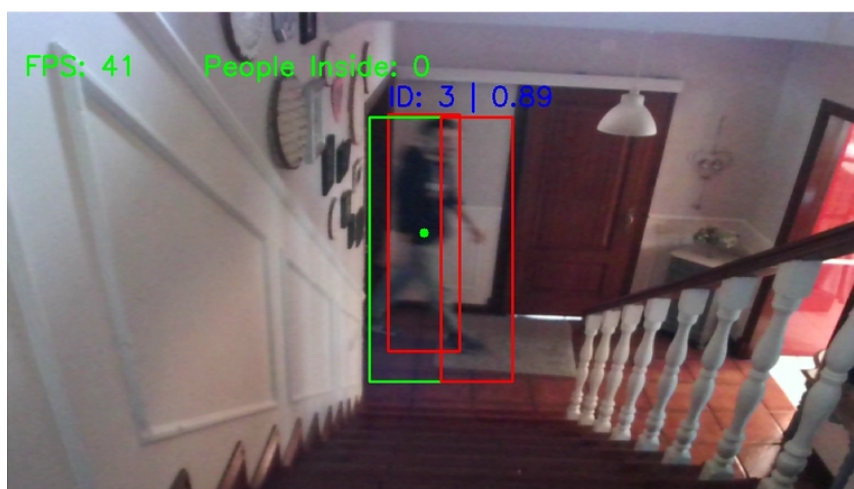
Figure 5.1: Live Video with YOLOv5 and DeepSORT, showing a count of 0 (using the X PyTorch model).
