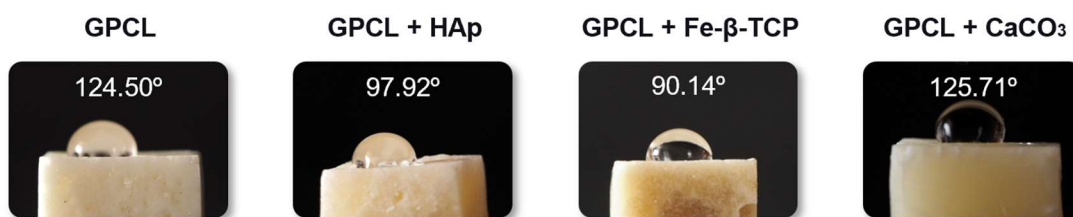
Figure 4.8 – Water contact angle of H 2 O droplet in each hydrogel.
