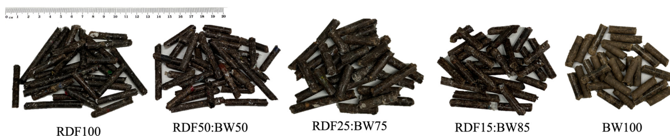
Figure 2. Pellets produced as a raw material for the slow pyrolysis process.
