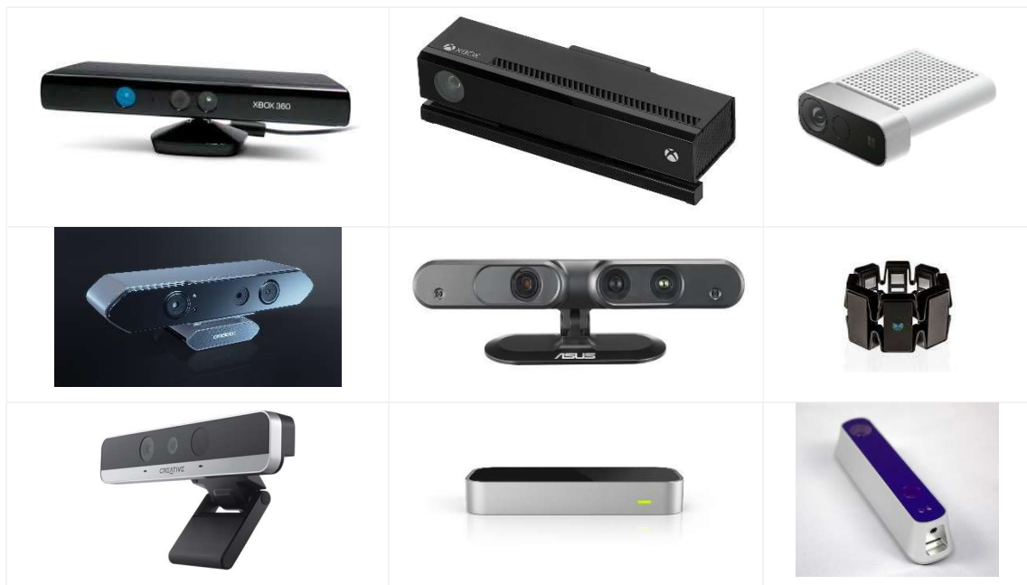
Figure 2 - NUI Sensors (from top left to bottom right: Microsoft Kinect v1, v2 and Azure; Orbbec Persee Astra; Asus Xtion; Myo; Real Sense D435; Leap Motion; and Structure)
