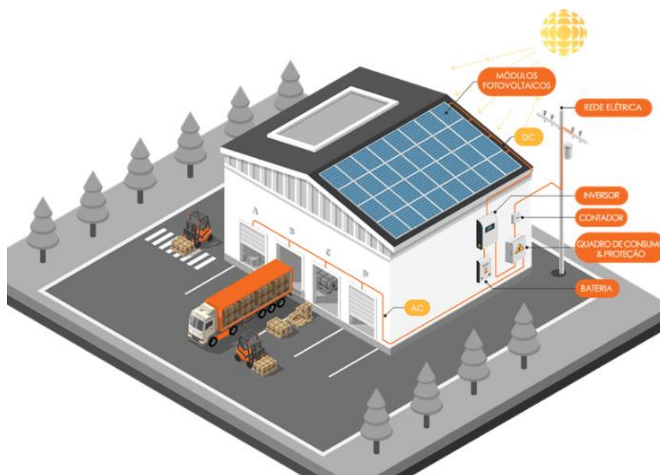
Figura 17- grid tie system (Sunenergy, 2022)
