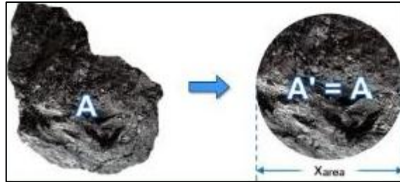
Figure 2.10 - Correspondence between area from a non-spherical particle and a spherical particle and x_{\text{area}} representation.
