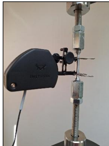
Figure 3.11 – Specimen with the clip gauge for the tensile test.
