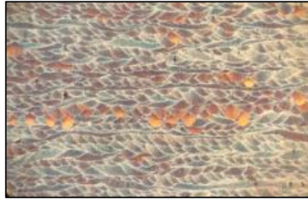
Figure 4.21 – Optical micrograph 50x magnification from a specimen etched with Keller's reagent for 30 seconds.
