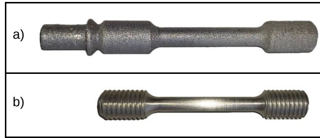
Figure 3.10 – Specimen a) as-built, and b) machined.
