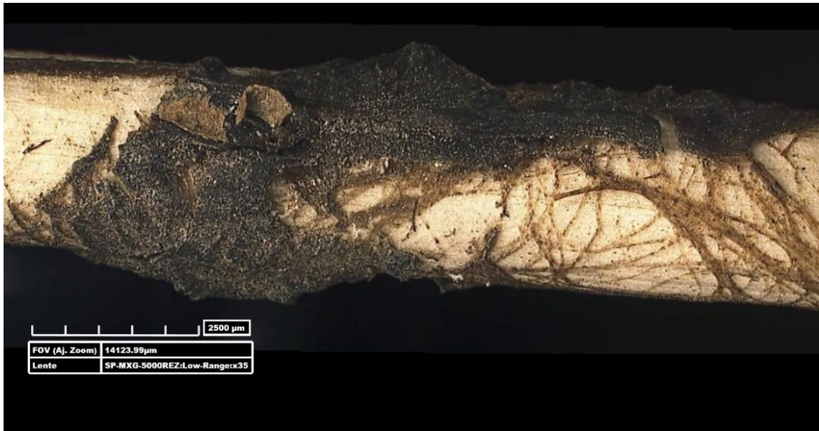
Figure 54: Details of the residues in algae fishing tool, SE_AF_19mar20_S1_T02). Taken at 35x.
