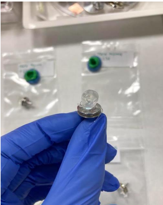
Figure 4.7 Pre-Treatment procedure set up at the Universitat Rovira i Virgili - scientific and technical resources Department. Example of positive cast (specimen n. “CC20_13/4_F8_52”) that has been separated from his negative mold and glued on a metallic stub. Photo taken by M. Mattera with an Apple iPhone SE of second generation (March 2023)
