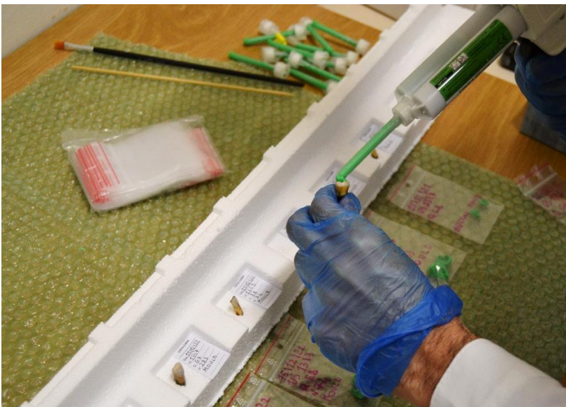
Figure 4.2 Photo of the Molding Process at the Paleoanthropological Lab. of Ferrara University. High resolution silicone is applied individually to each specimen using a gun dispenser, teeth are placed back into the polystyrene slab at the end of the process. Photo taken by J. Arnaud with a reflex camera Nikon D3100 (December 2022)
