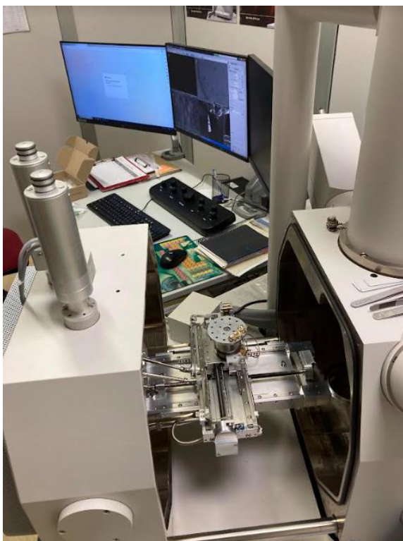
Figure 4.9 Observation process of Ciota Ciara's dental casts using ESEM microscope at the Universitat Rovira i Virgili - scientific and technical resources Department. Photo taken by M. Mattera with an Apple iPhone SE of second generation (March 2023).
