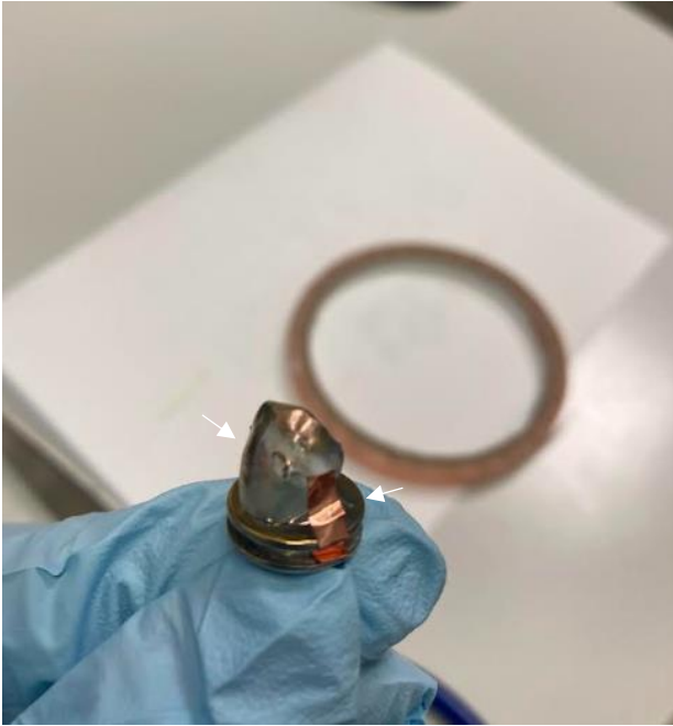
Figure 5.8 Example of the cast specimen n. CC20_13/7_G7_283 (canine) after the application of a metal tape (copper) (white arrows). This process will help for a proper surface spread of the electron beam in the SEM chamber. Photo taken by M. Mattera with an Apple iPhone SE of second generation (March 2023).
