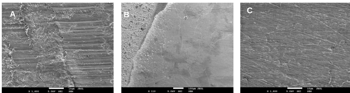
Fig.3- A) SEM image of Group B Enamel surface after remnant adhesive removal with tungsten carbide bur: horizontal risks are formed within the horizontal grooves. Some unpolished areas can be observed as a result of smear layer deposition. B) SEM image of Group C Enamel surface after remnant adhesive removal with Sof-Lex™ polishing discs: polished remnant adhesive is present on the left side, and a thin remnant adhesive layer with an homogeneous smooth appearance is formed in areas where nearly all adhesive was removed (right side). C) SEM image of Group C Enamel surface after remnant adhesive removal with Sof-Lex™ polishing discs: polished surface is present with small risks dispersed all over the enamel.
