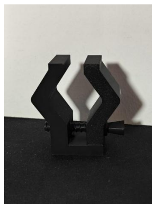
Figure 6.1 – 3D-printed support for laser that can be attached to a tripod
