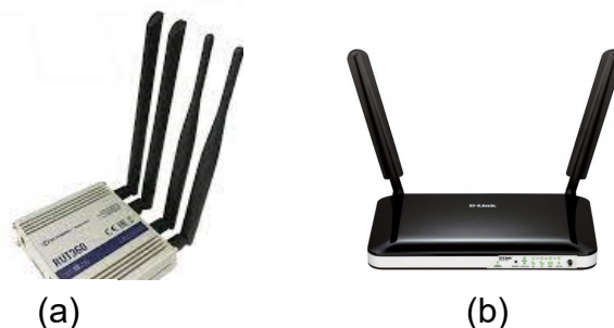
Figura 45 – Routers 3G/4G escolhidos para o Sentry: (a) RUT360; (b) D-link DWR-921
