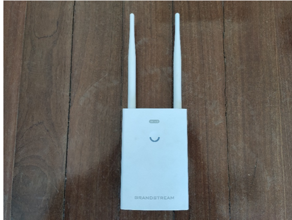
Figura 3.2: Access Point Grandstream GWN7660LR.
