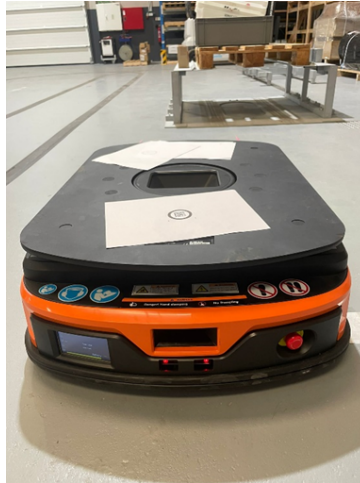
Figura 3.10: AMR HIKROBOT MR-Q3-600LE-DI(CE).
