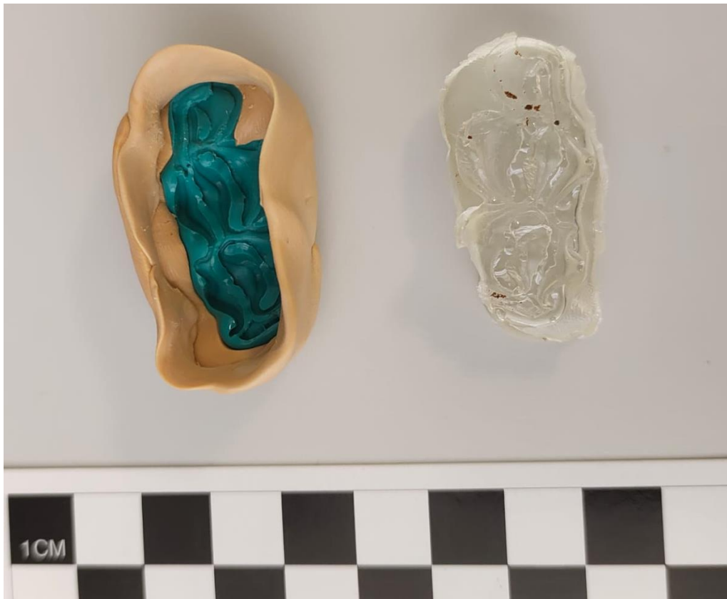
Figure 9. The silicone mould (left) and resin replica (right) of the specimen RT6417
