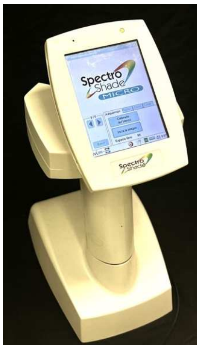
Figura 21. Espectrofotômetro Spectro-Shade Micro (MHT - Niederhasli, Switzerland).
