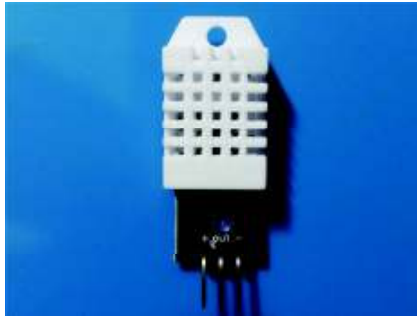
Figure 4.3: DHT22 sensor used in the smart agricultural cabinet
