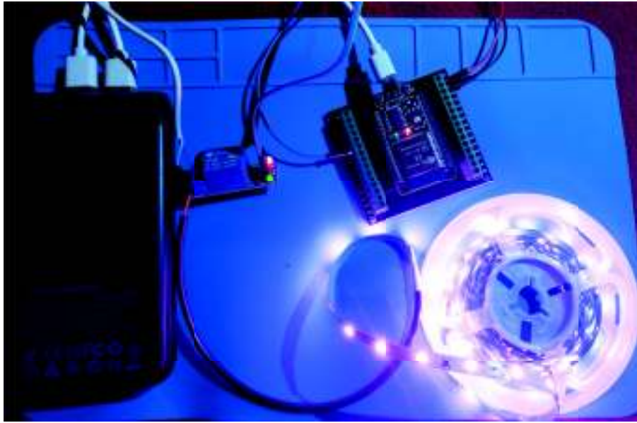
Figure 4.11: Lightning system assembly
