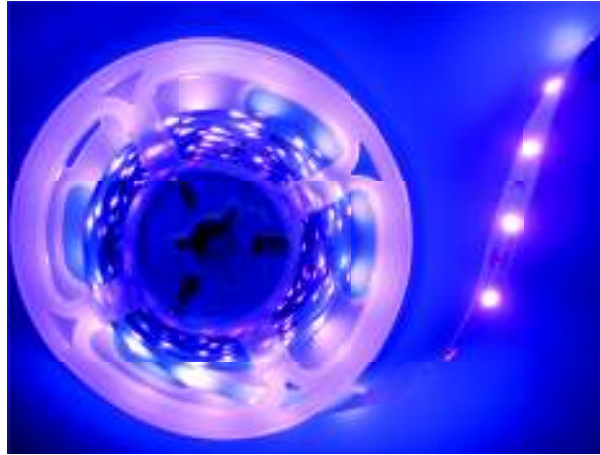
Figure 4.6: Phytolamp used in the smart agricultural cabinet
