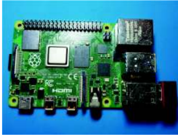
Figure 4.1: Raspberry Pi 4 model B used in the smart agricultural cabinet
