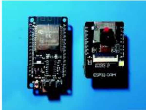
Figure 4.2: ESP32 and ESP32-CAM used in the smart agricultural cabinet
