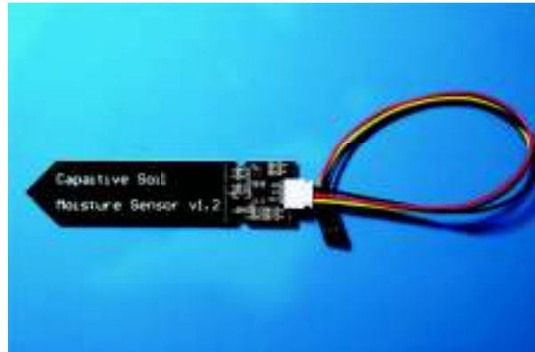
Figure 4.4: Soil moisture sensor used in the smart agricultural cabinet
