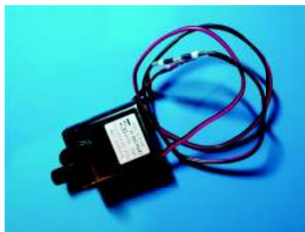
Figure 4.5: Water pump used in the smart agricultural cabinet
