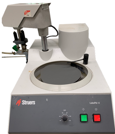
Figura 22 - Polidora (LaboForce-1, Struers, Denmark).
