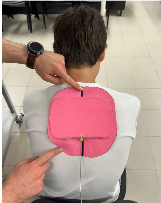
FIGURE 4.17: Experimental Test with the WPPA covered by neoprene and a Human Body
