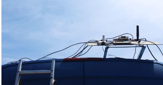
Figure 4 – Structure used to secure the cameras to the mobile platform with sensors 01 and 02 attached.
