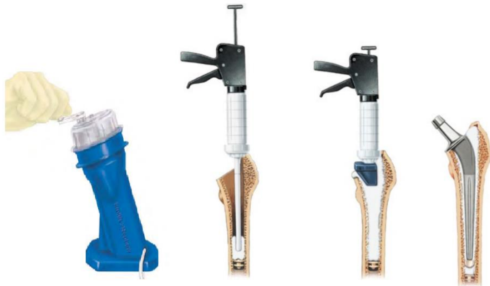
Figure 2.8 - Schematic representation of a third-generation cementing technique (Smith and Nephew, n.d)
