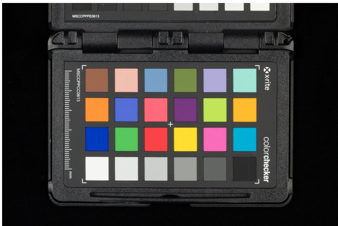
Fig. 25 – mira de cor X-Rite ColorChecker Passport
