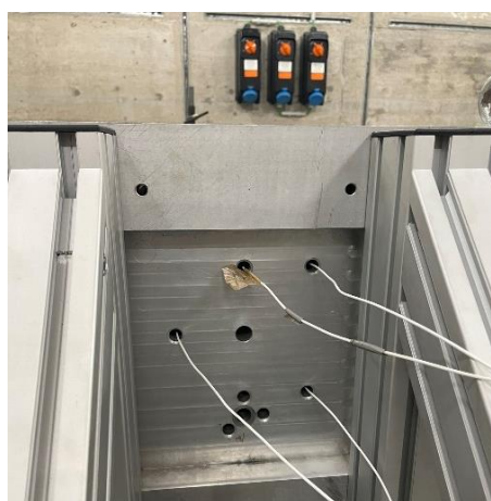
Figure 53: Backside of the reaction plate with sensors in place
