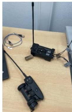
Figure 55: Breach MC system - remote firing device (Breach MC RX-ST) connected to the PXIe Platform at the top and the transmitter controller (Breach MC TX) at the bottom of the picture
