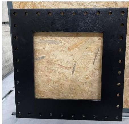
Figure 70: 10 mm thick mobile steel plate
