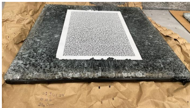
Figure 105: Laminated glass after removal from the structure
