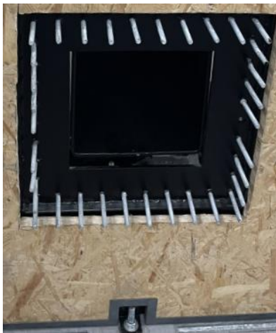
Figure 69: Steel frame with threaded rods with the shock tube in the background
