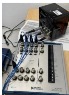
Figure 57: Data acquisition system NI6361 and the Photron FastCam mini AX100 at the top
