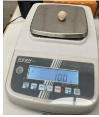
Figure 48: 10g of PE-4A weighed on a precision balance
