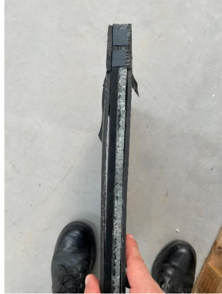
Figure 95: Lateral view clearly showing the difference between the shattered outer ply and the intact inner ply, with rubber bands still attached
