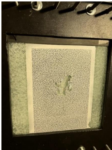
Figure 99: Laminated glass attached to the structure after the test, outer ply shattered
