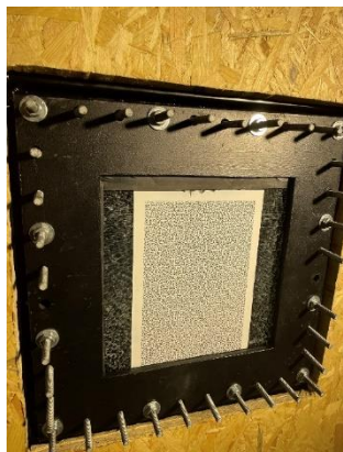
Figure 104: Laminated glass attached to the structure after the test
