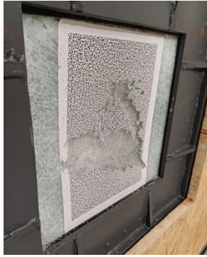
Figure 81: Laminated glass attached to the structure after the test
