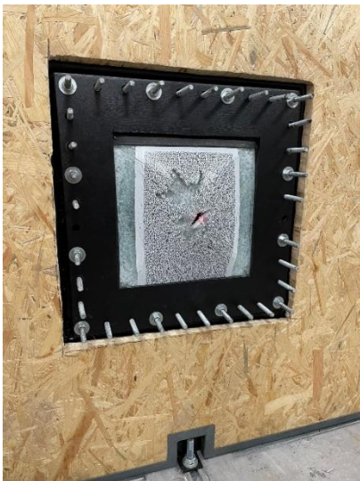
Figure 96: Laminated glass attached to the structure after the test, with a hole going through all layers
