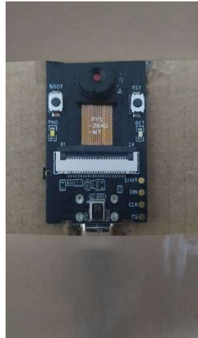
Figure 113 – Camera fixed inside the prototype.
