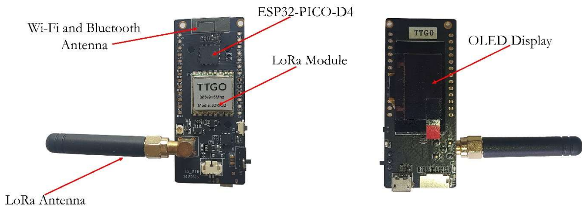
Figure 40 – Rear and frontal view of the LoRa32 T3 model.
