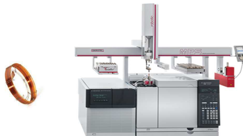
GC HP 7890A GC coupled to 7000B MS/MS detector
