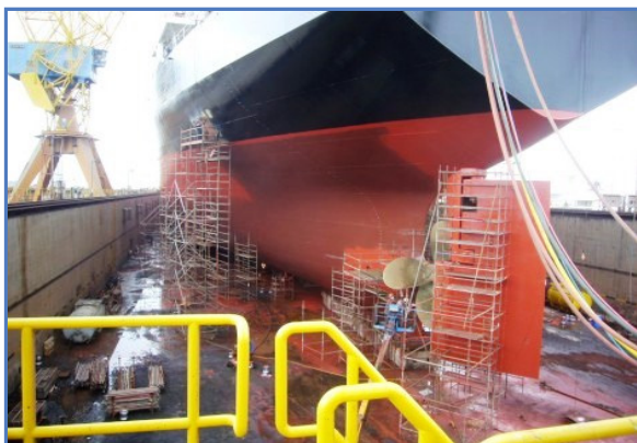
3 PS, aft. Application of 2nd full coat of A/F red on Boottop
