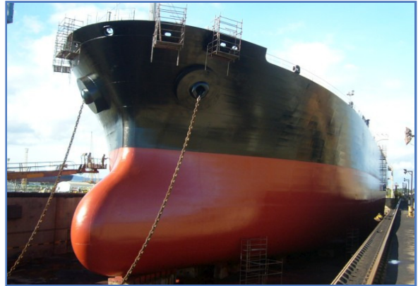
8 PS general view from fore after completion of last full coat of A/F.
