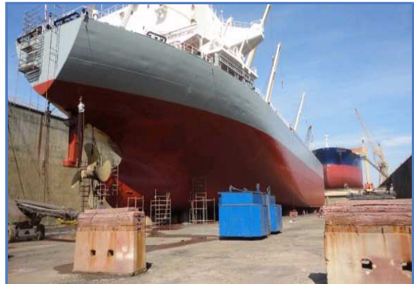
26 Toside finishing coat 56360 Grey 11480; Boottop finishing coat 5636 Red 50630 and AS/F Olympic 86950 Red 51110.
