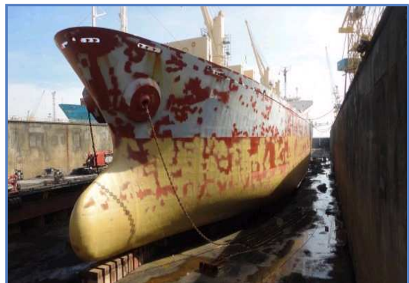
22 PS-Topside: 2sd touch ups Hempatex HB 46410 Red 50630; B/T + V.B. 2sd touch ups Hempadur 45182 Yellowish Grey 25150 (sealer coat).
