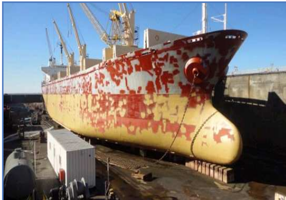
25 SBS-Amount of primer prior to finishing coats.
