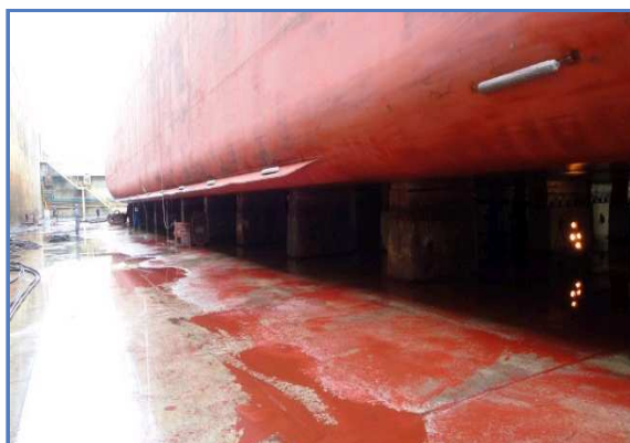
12 PS-After HPFWC (A/F leach layer on the ground).
