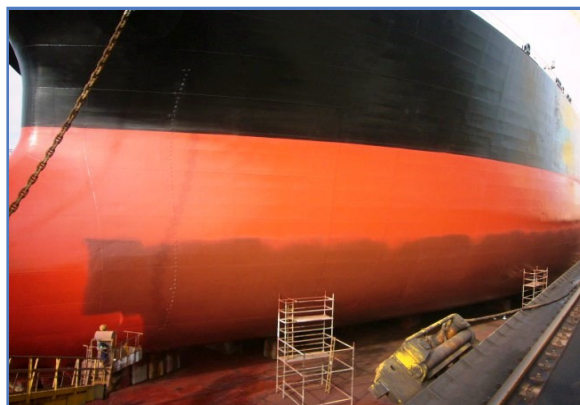
4 PS, fore. Application of 2nd coat A/F red on Vertical Bottom
