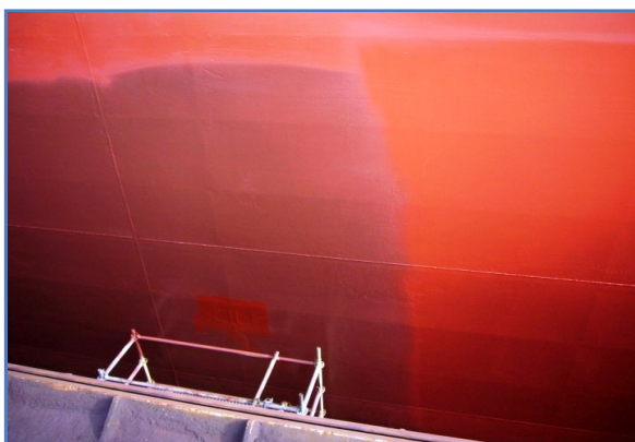
5 SBS. Application of 2nd A/F full coat. A treated marked area can be observed after application of 1st primer coat Hempadur Quattro red by roller.
