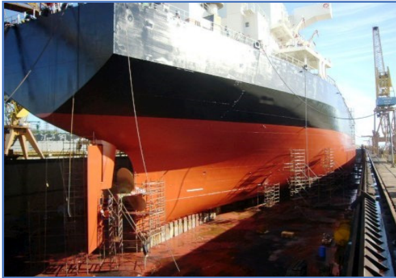
7 SBS, aft. Completion of last full coat.
