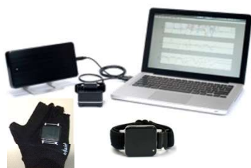
Fig.1 Mobility Lab System with Opal Accelerometer
