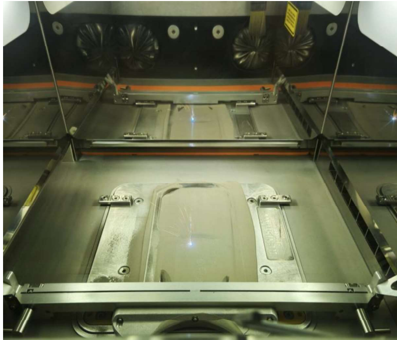
Figure 3.3 - Cylinders with porous structure being produced by L-PBF.
