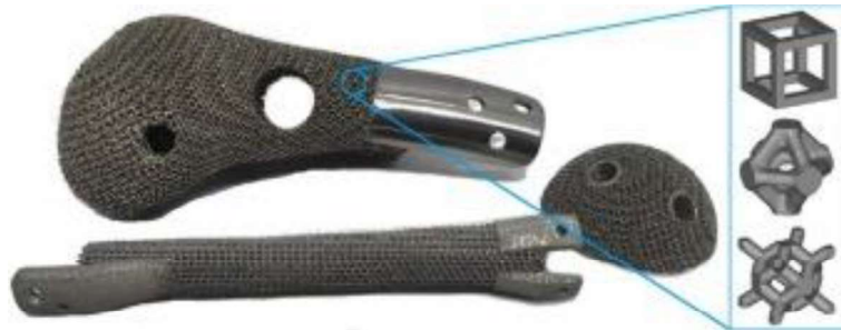
Figure 2.10 - Implants of titanium with controllable structural units fabricated by laser powder bed fusion (L.-C. Zhang et al., 2023).
