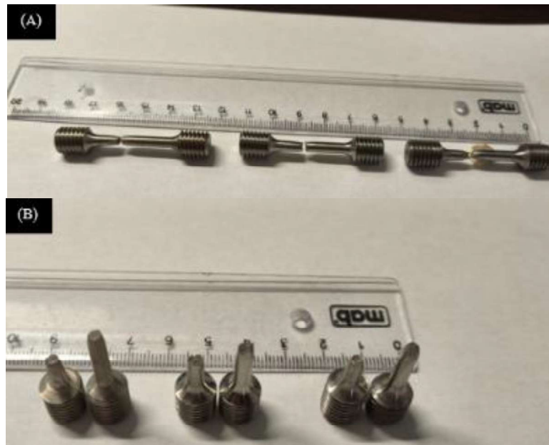
Figure 3.9 – Fractured tensile specimens: (A) horizontal build and (B) vertical build.
