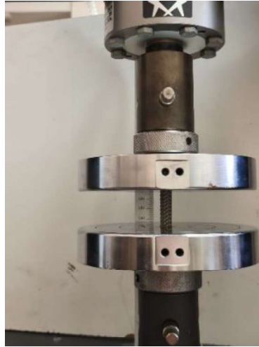
Figure 3.8 - Compression test of a cylinder with gyroid structure on the Instron 3369 universal testing machine.
