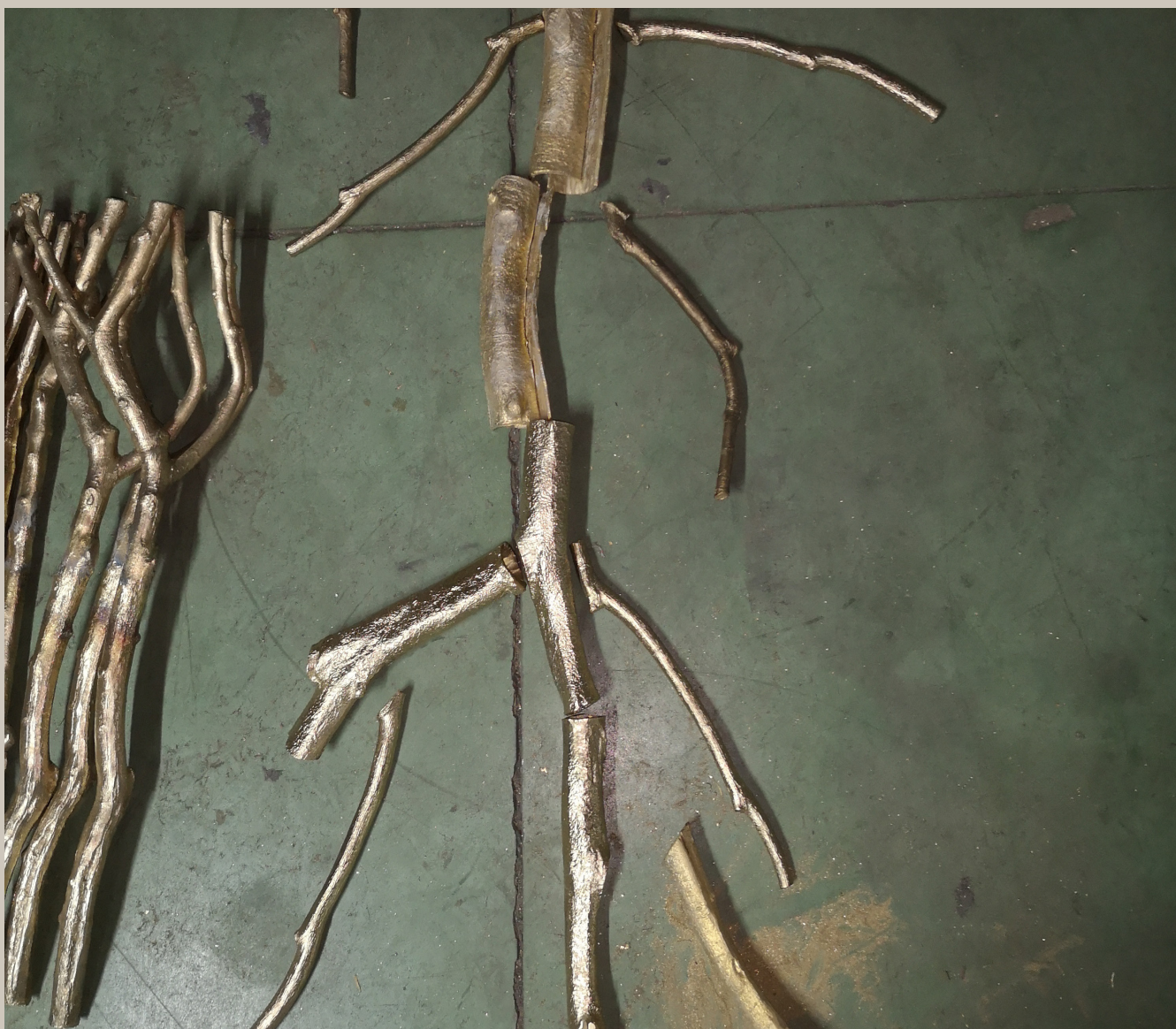
2.10. Final piece shape after hand casting
