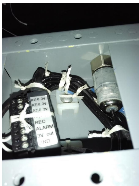
Figure 6 – Schematic of the electrical connector and pressure switch.
