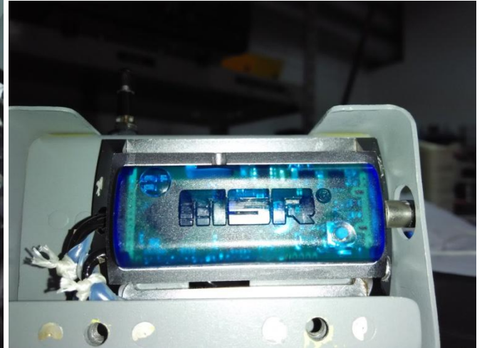
Figure 8 – MSR 165 and cables installation.
