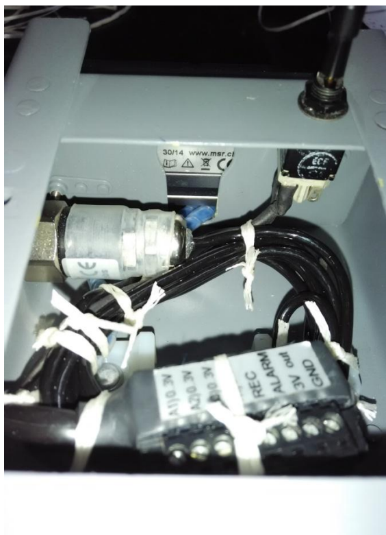
Figure 7 – Detail of the switch installation and the cover used to protect the cables from chafing.
