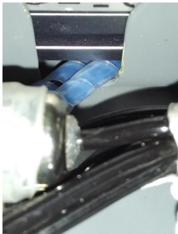
Figure 7 – Detail of the switch installation and the cover used to protect the cables from chafing.
