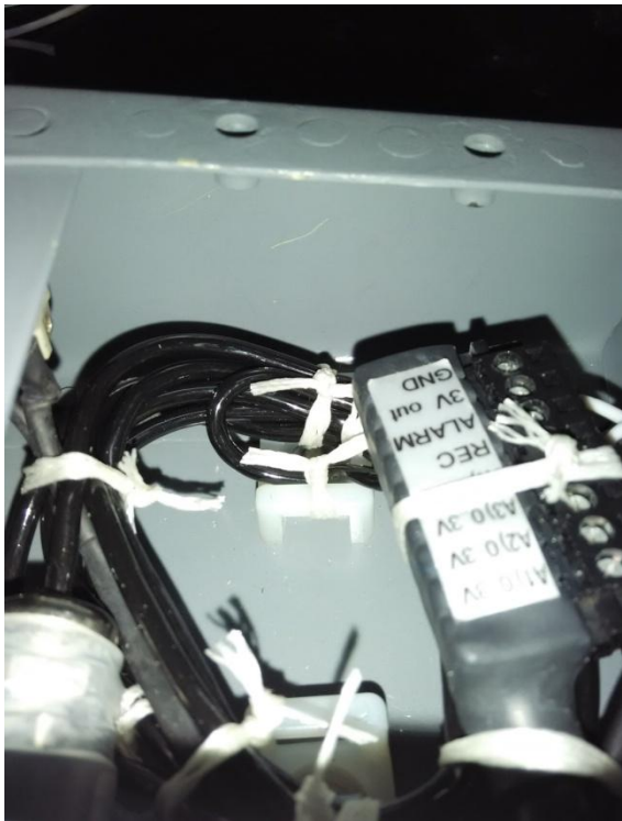
Figure 8 – MSR 165 and cables installation.
