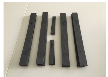
(d) Some specimens after being milled and sanded.
