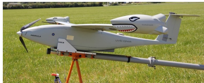
(b) N1 with wing tip pods installed
