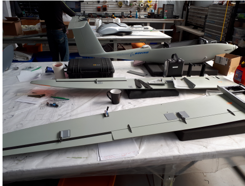
Figure 2.10: N1 disassembled at UVic CfAR' shop
