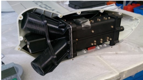
(a) MSU mounted inside the pod
