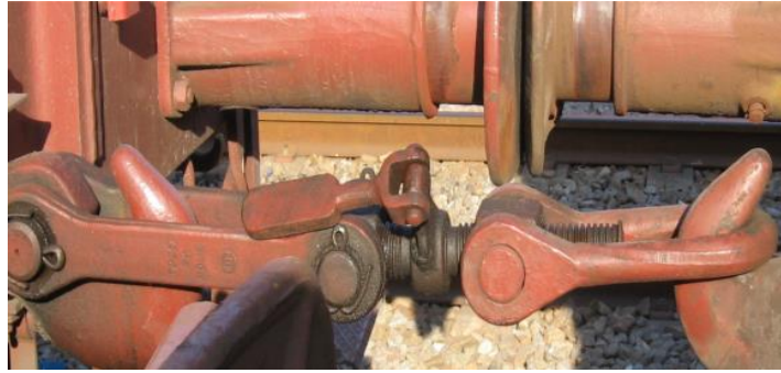
Figure 3 – UIC standard coupling system (source: IET 51 IMTT).
