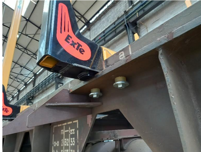
Figure 51 – Timber bunk fastened with rubber pucks.
