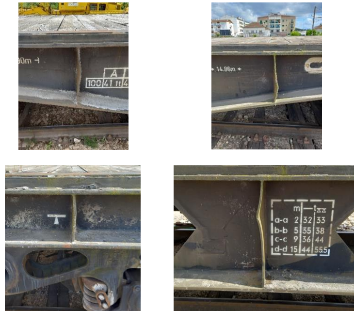
Figure 43 – Deformation regions identified in the chassis.
