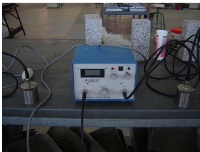
Figura 70. PUNDIT (Portable Ultrasonic Non Destructive Digital Indicating Test).
