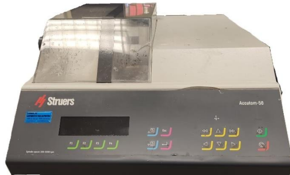
Figura 5. Micrótomo de tecidos duros (Accutom-50, Struers A/S, Ballerup, Denmark)
