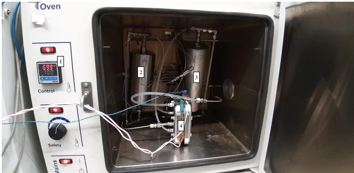
Figure 12- Open oven: 1- Oven control interface; 2- Anode Bubbler; 3- Cathode Bubbler; 4- Fuel cell
