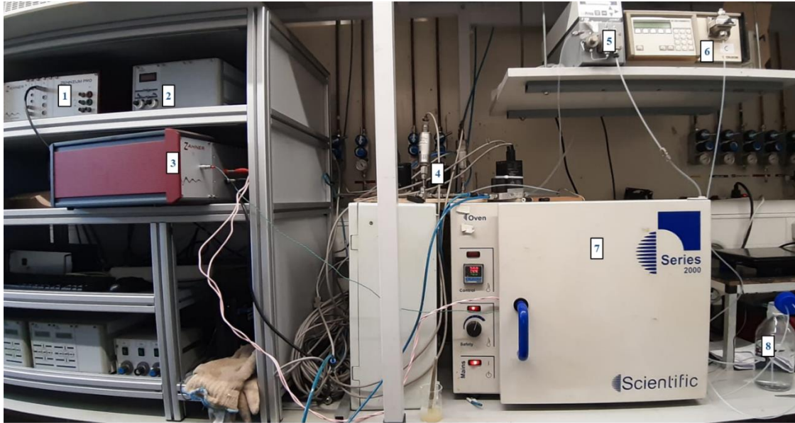
Figure 11- Test bench overview: 1- Zenium PRO potentiostat; 2-Additional control box; 3-PP241; 4- Flow and Pressure controller board; 5- Anode HPLC pump; 6- Cathode HPLC pump; 7- Scientific oven series 2000 for cell temperature control; 8- Water deposit
