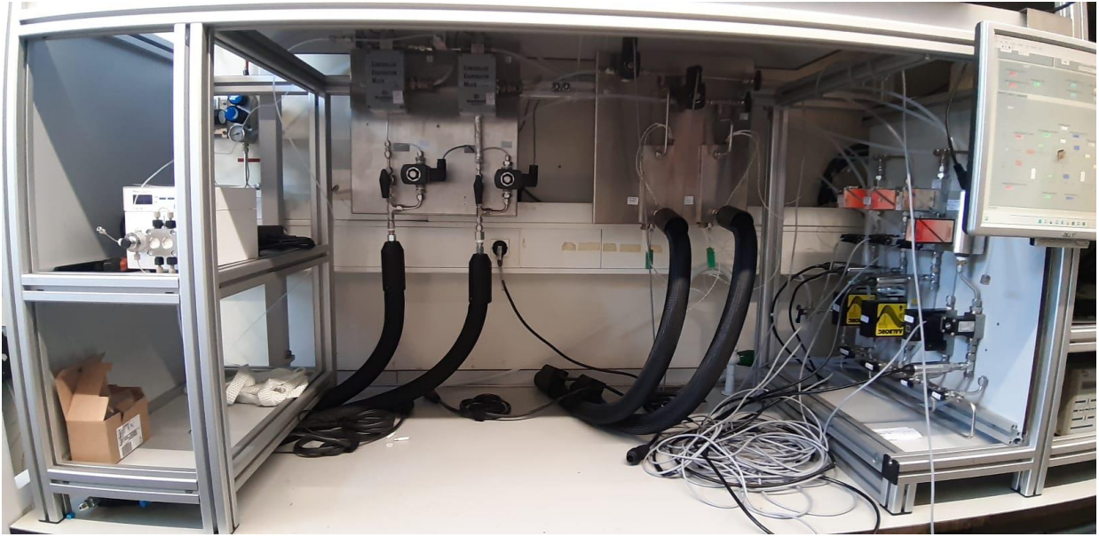
Figure A- 2 - Test bench that is being assembled in FEUP for testing both fuel cells and electrolyser
