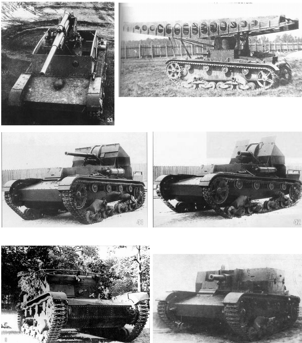
Figure 9 The T-26 “family” of vehicles. From the top, left to right, SP AA Gun; Bridge Layer, SP Gun, SP Howitzer, Command Post Vehicle and Assault Gun. The Soviets introduced in the 30s the “combat team” concept adopted by the US in the 40s. This advanced concept was abandoned after Tukhachevsky’s death, and next generation tanks, such as the 1940 T-34 were not built according to this principle, assault gun and tank destroyer variants only being introduced in 1943.
