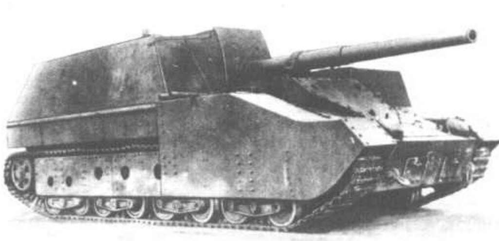
Figure 10 A Su-14-2 152mm Self-propelled Gun. The soviets experimented intensively with self-propelled artillery in the 30s, including heavy weapons in corps artillery calibers.
