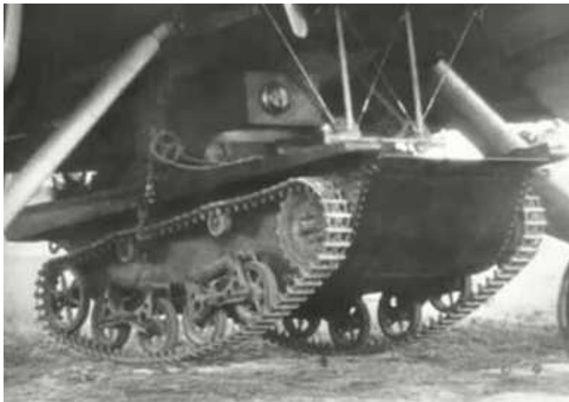
Figure 4 A T-37 tankette slung under a TB-3 Bomber for air deployment. Tukhachevsky ideas for mechanizing airborne units led to extensive experimentation.
