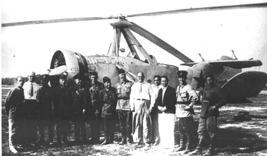
Figure 13 A Kamov A-7 autogyro, the world’s first autogyro designed for armed combat missions, it could perform very short take off and near vertical landings. (Gunston, 2000).
