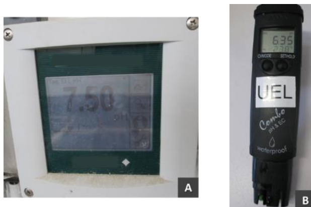
Figure 27 – Equipment used to measure pH. A – Equipment linked to a probe and a signal convertor that measures pH and temperature; B – Portable pH meter.
