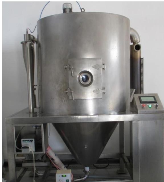
Figure 33 – Spray Dryer at UEL.
