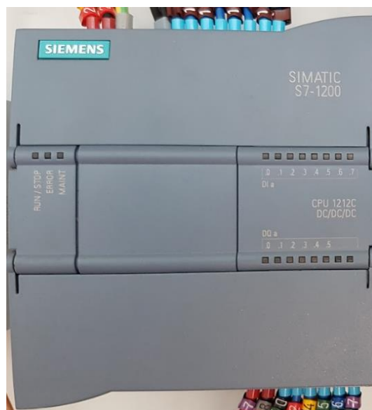
Figura 47 – PLC Siemens S7-1200
