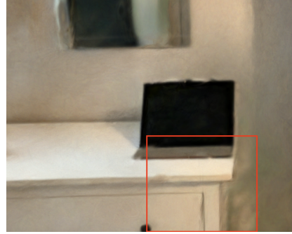
(b) OpenSplat output for just wide lenses, showing in detail straight lines less harmed by undistortion interpolation
