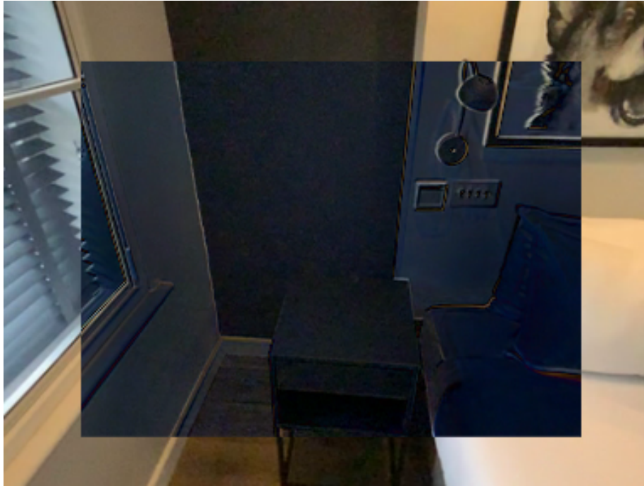
Figure 17: Overlaying comparison between final preprocessed ultrawide image and original wide image, with the overlapping FOV applied with a difference blend mode and the extra FOV still present after undistortion and cropping represented normally, as a frame to the wide image.
