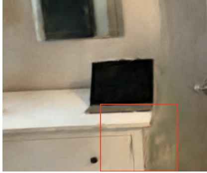
(a) OpenSplat output for both lenses, showing in detail the tunneling effect resulted from undistortion interpolation
