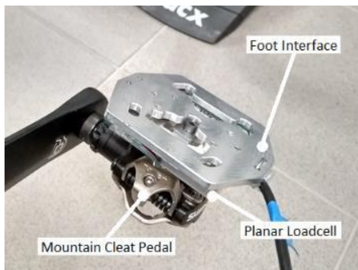
Figure 2.4 – Instrumented Pedal Device.
