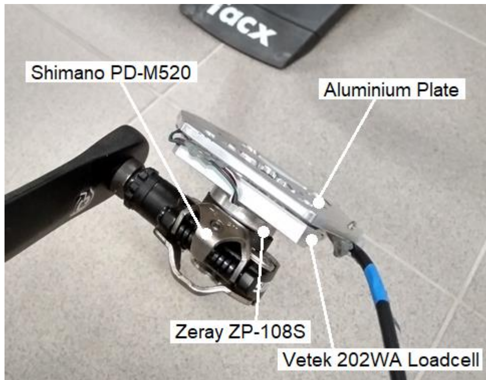
Figure 3.43 – Instrumented Pedals Device installed and with legend
