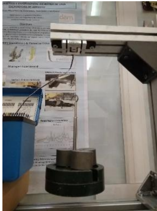
Figure 3.57 - Vetek 202WA calibration laboratory setup
