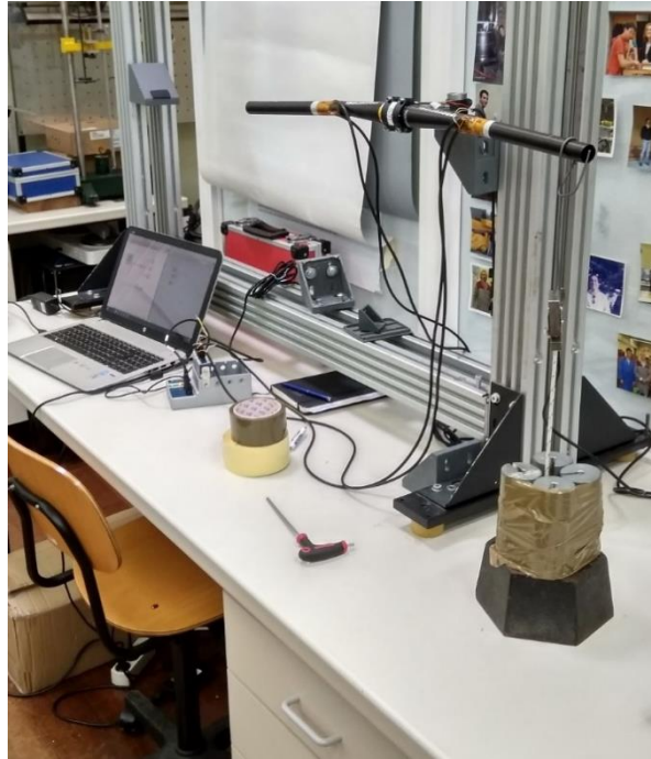
Figure 3.40 - Strain gauges calibration laboratory setup
