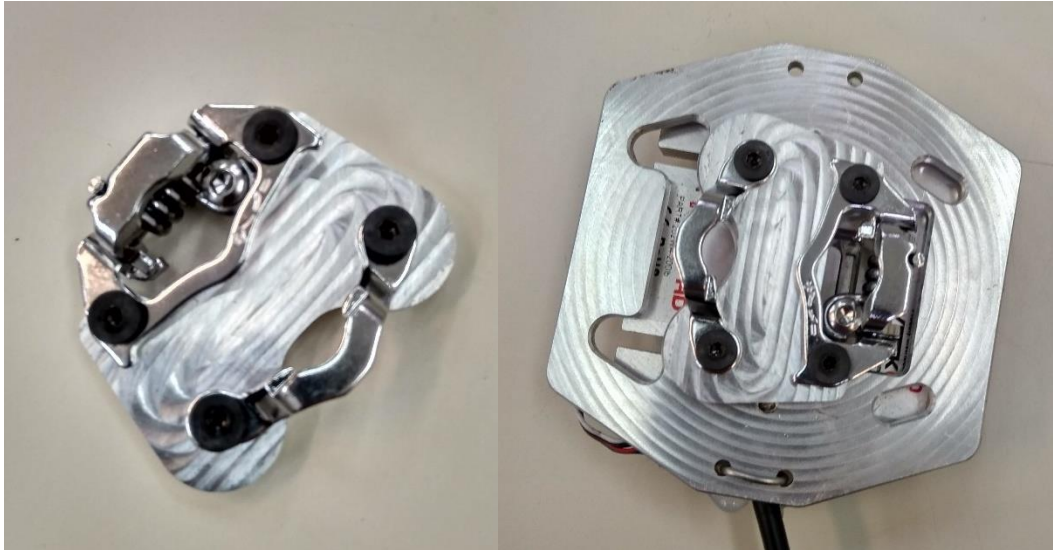
Figure 3.44 - Clipping Shoe Interface on the left and the Clipping Shoe Interface installed on the Foot Interface on the right
