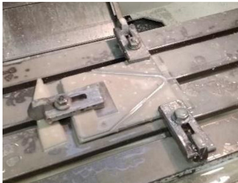
Figure 3.29 – Waste pieces clamped to the worktable
