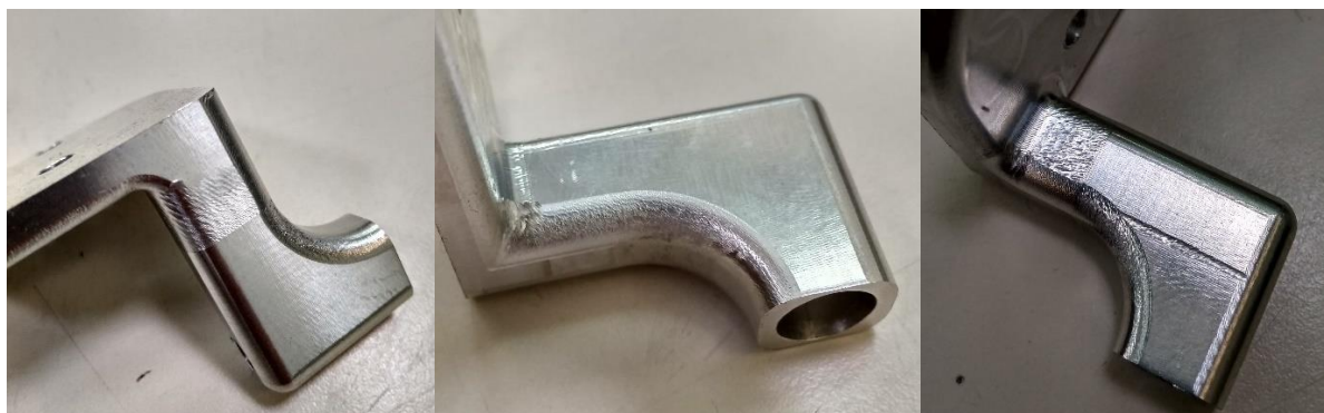
Figure 3.32 - Tool vibration imperfections
