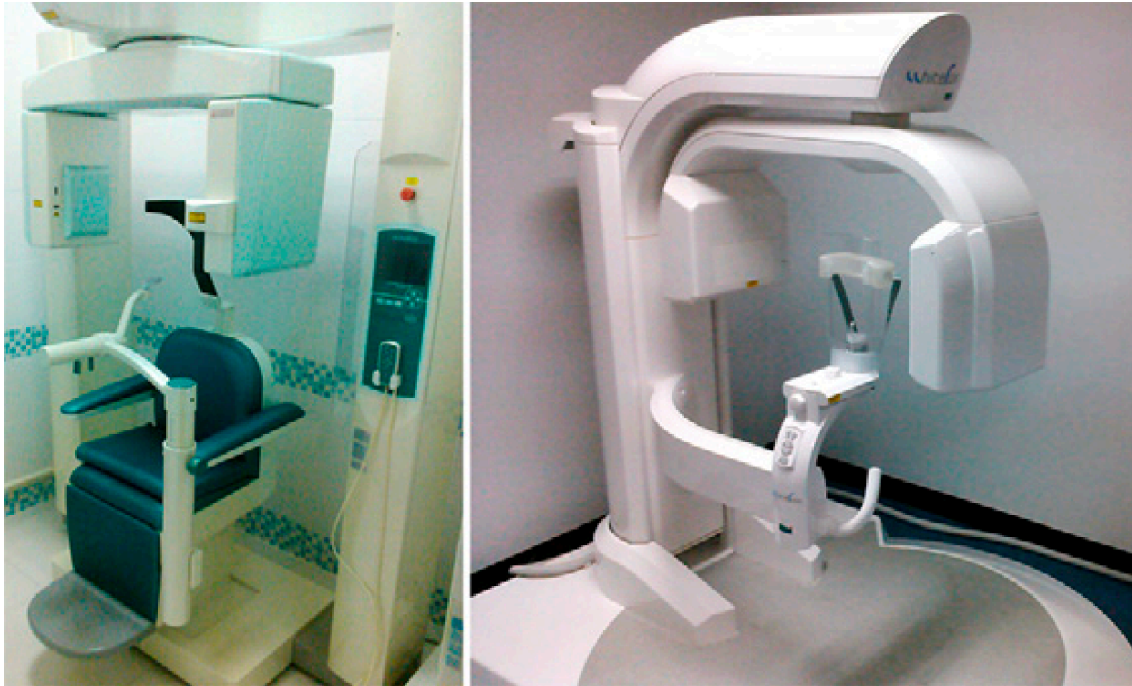
Figure 22: Different types of CBCT gantries. Left: seated patient position (3D Accuitomo® 170; J. Morita, Kyoto, Japan). Right: standing patient (WhiteFox®; Acteon Group, Merignac, France)
