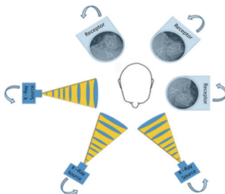
Figure 7 : CBCT, Principle of basis image acquisition where in X-ray source and Image receptor reciprocate around patient 180 – 360 degrees to acquire 2D cephalometric images (Venkatesh & Venkatesh Elluru, 2017)
