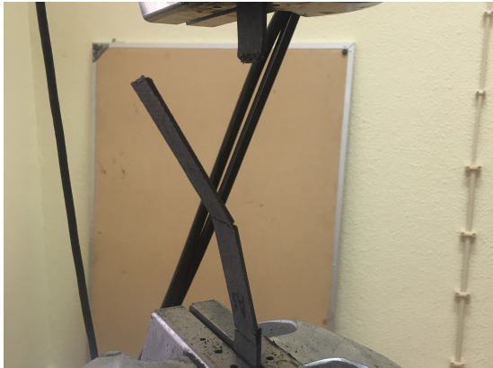
(b) Bidirectional specimen breaking in three different points.
