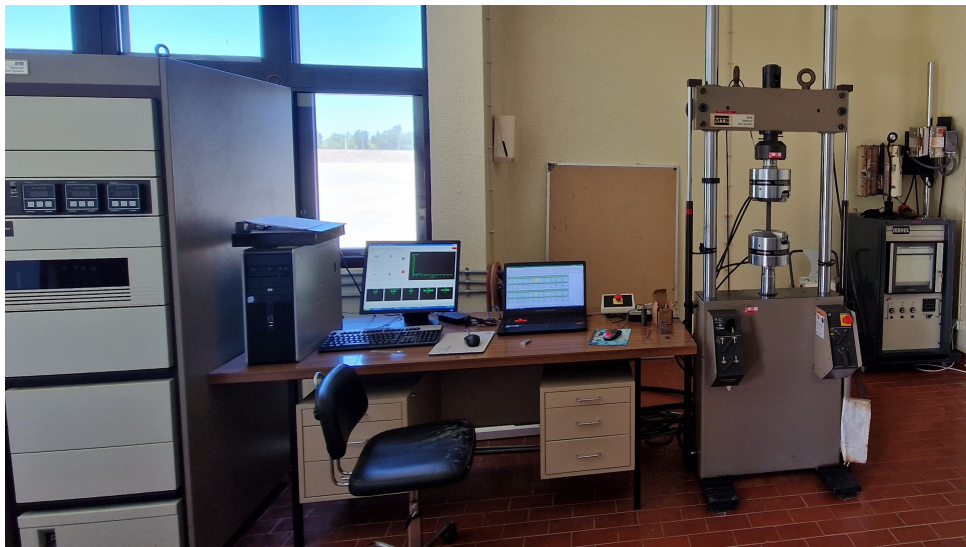
Figure 3.6: Tensile testing machine and its computers.
