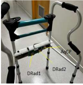
Fig. 3. Smart Standard Walker Prototype including two microwave radars (DRad1 and DRad2) and acquisition and communication platform (AqCP).
