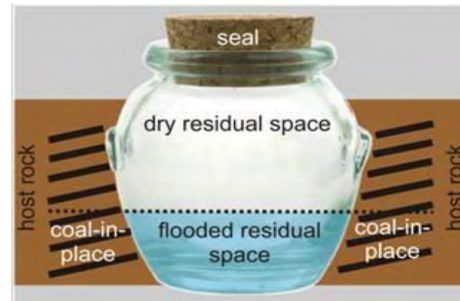
Figure 8 – The different elements of the jar pot model, with partially flooded residual space corresponding to the jar (Piessens 2012).
