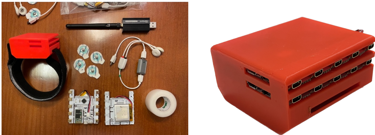
Figure 19. Data acquisition materials (left) and 3D printed case (right).
