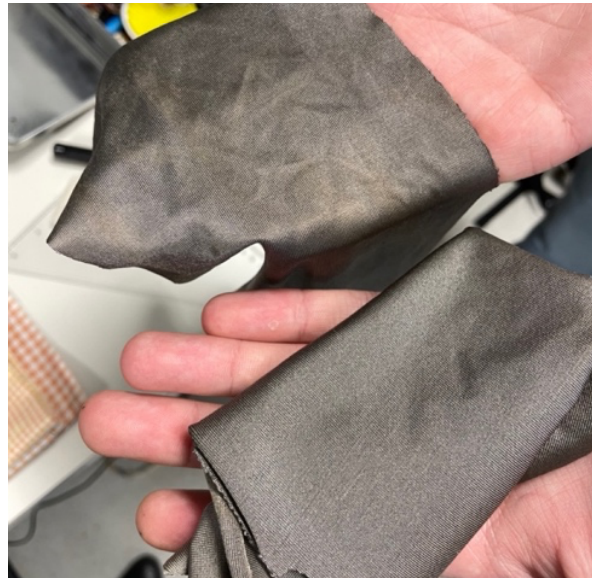
Figure 14. Conductive lycra. Discoloured from oxidation (top).
