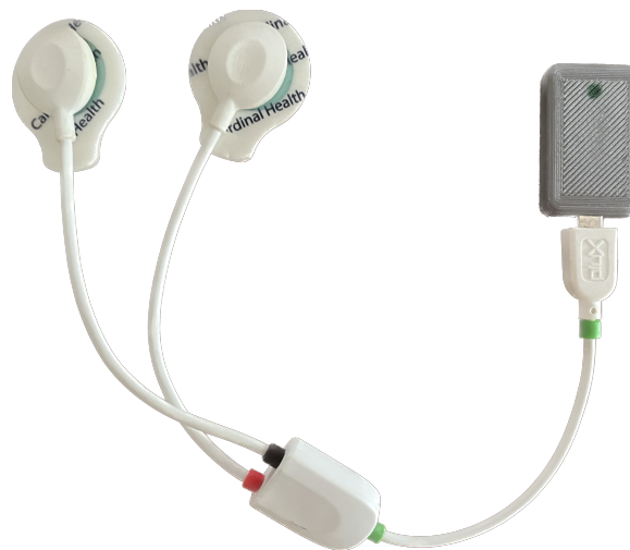
Figure 2. EDA sensor (PLUX) connected to hydrogel electrodes (Cardinal Health).
