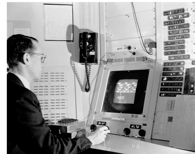
Figura 5: IEEE Spectrum (2023). Ivan Sutherland developed the computer drawing tool Sketchpad for his Ph.D. thesis [Fotografia]. IEEE Spectrum. https://spectrum.ieee.org/sketchpad .
