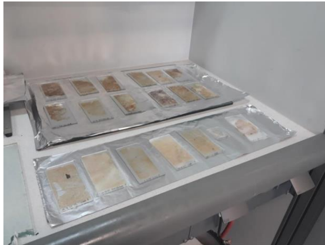
Figure 9: Final Thin section of a thickness of 30 micron (Photo-Opeyemi Adewumi, 2019)
